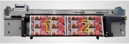
It can print two rolls of 1.52M media together to save more time, labor work and workspace
