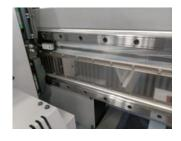
Adopt metal raster with magnetic linear motion sytem, higher printing resolution and stability with longer lifespan
