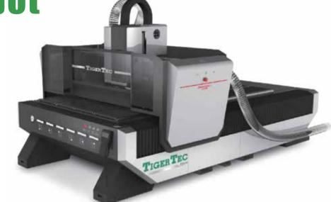
TigerTec TR408 Robot is a totally new designed product which is mainly used for wood processing. Heavy welded table and gantry are applied in this type for better stability and accuracy. The machine is driven by servo driving system for high travelling speed. A 9 kw HSD aircooling spindle is used for this machine. There are 6/8/12 pieces tool holders for changing the tools easily.
