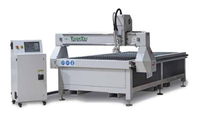
TigerTec TR408P is the best choice and easy to use cutting plasma machine. In standard we use Hypertherm power generator from USA. Any other brand of generator can be used on request. The machine is equipped with a stand-alone controller that can process files from different CAD CAM software. It's equipped with height control to ensure a good cutting even on non-flat surfaces.
