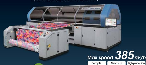
16 printheads arranged in two staggered lines
